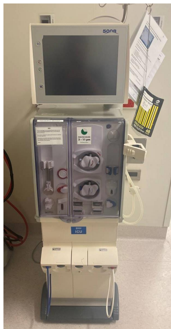
Image 1 : Fresenius 5008 RRT system. The machine is directly connected to a reverse osmosis purifier which generates the large amount of dialysate needed for HV-CVVHDF. Spent ultrafiltrate and dialysate is plumbed directly to the sewerage negating the need for dialysis bag changes.
